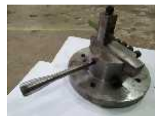
Figure 4.6 Instal toolholder on the upper tool post
