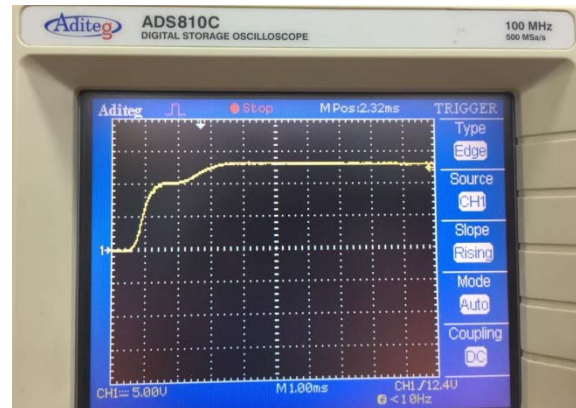
Fig. 4.11 Closed loop response output buck converter with controller
