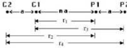
Figure 1. Structure of Dipole-dipole electrode configuration.
