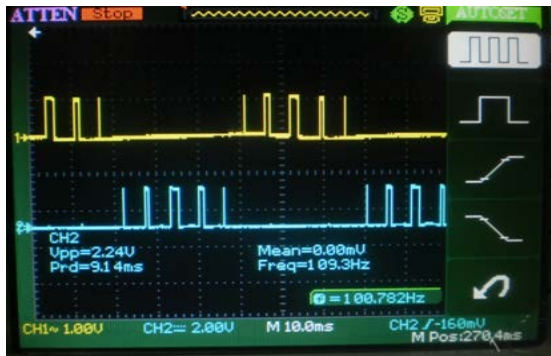
Figure 4. PWM pulse oscilloscope photograph of real measurements
