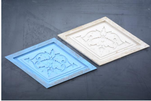
Figure 1 Mold is made of silicone rubber
