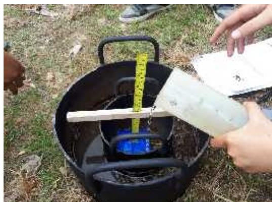
Pengisian Air Pada Ring Infiltrometer
