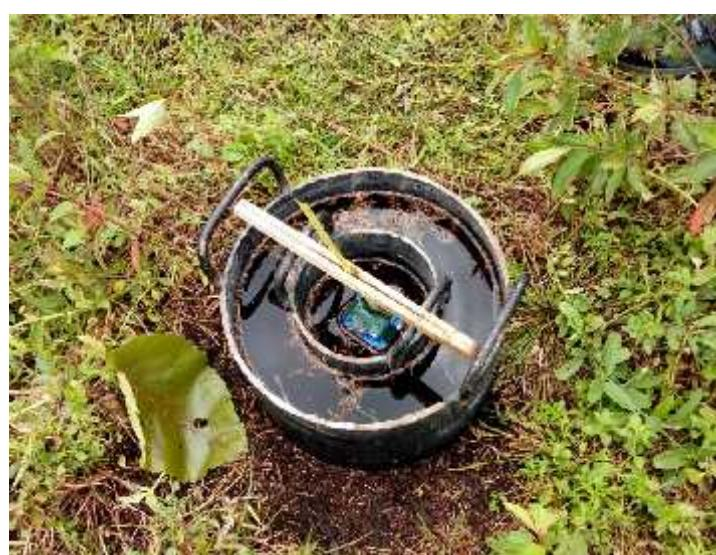
Gambar 2. *Double Ring Infiltrometer*
